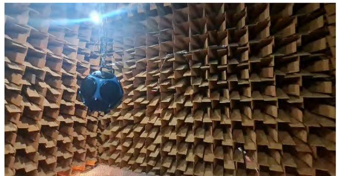
Figure 1: Speaker mounted in anechoic chamber with traversing microphone.
