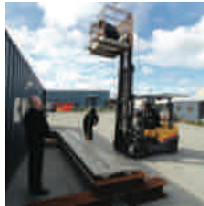
Figure 9: Impact testing of a panel from 3 m
