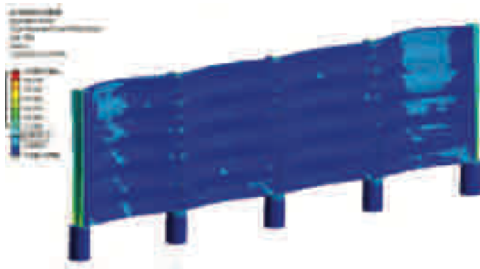
Figure 6: Stress distribution for model exposed to 150 km/h steady wind load
