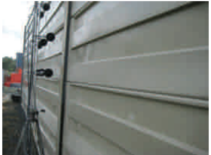
Figure 2: Microphone array in position for in-situ testing
