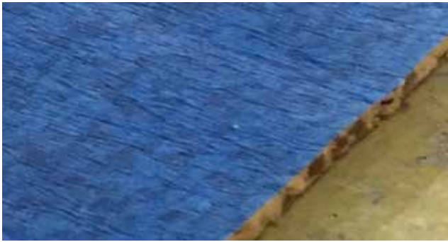
Figure 5: 10mm foam underlay with plastic coating
