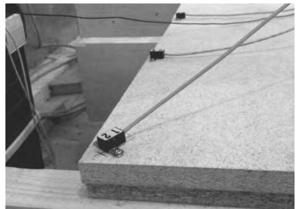
Figure 6: Array of accelerometers along the borders.
