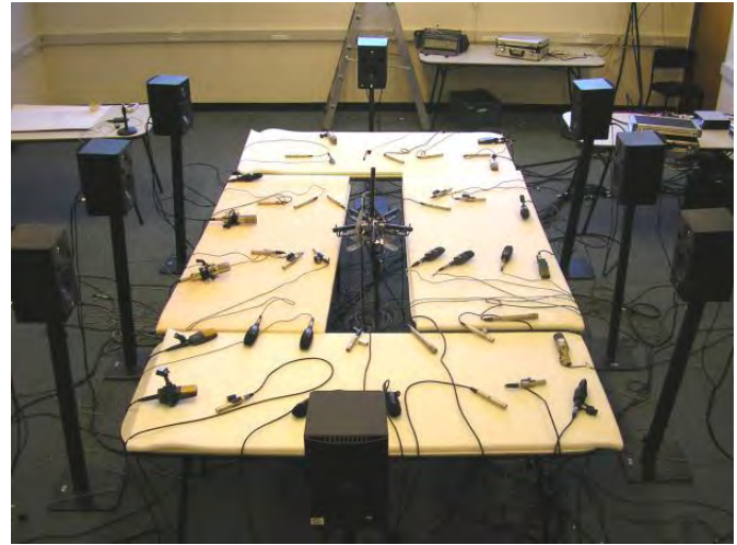
Figure 4. The final layout corresponding to recording 10 in Table 1, with all 48 microphones in place.
