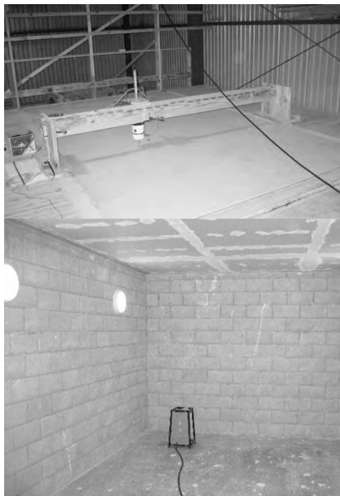
Figure 1. An electrodynamic shaker (top) and setup of the laser vibrometer to measure the ceiling (bottom).
