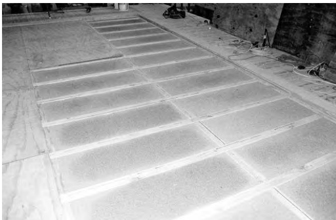
Figure 8. Top: RMS velocity comparison between sand-sawdust and sand-only upper layer. Bottom: Photo of sand-sawdust layer before plywood cover.
