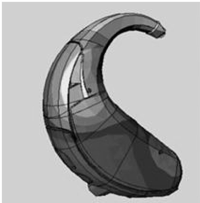
Fig.11. Left: Conformal sound intensity map on a hearing aid at 2400Hz. Right: refined beamforming sound intensity map on wind turbine at 4000Hz
