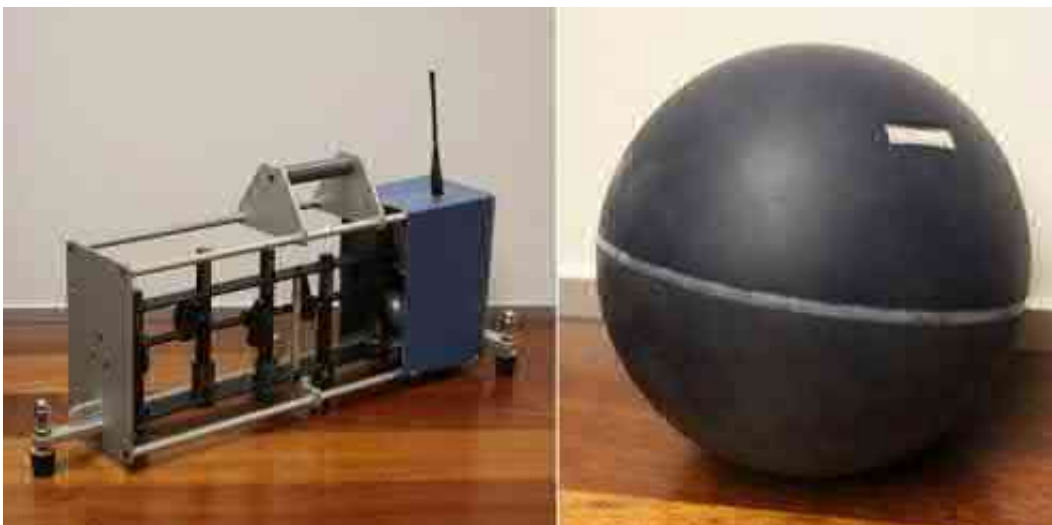
Figure 1 – Tapping machine (left) and standardised rubber ball (right) used during floor impact testing. Norman Disney & Young (Tim Beresford, 2018)
