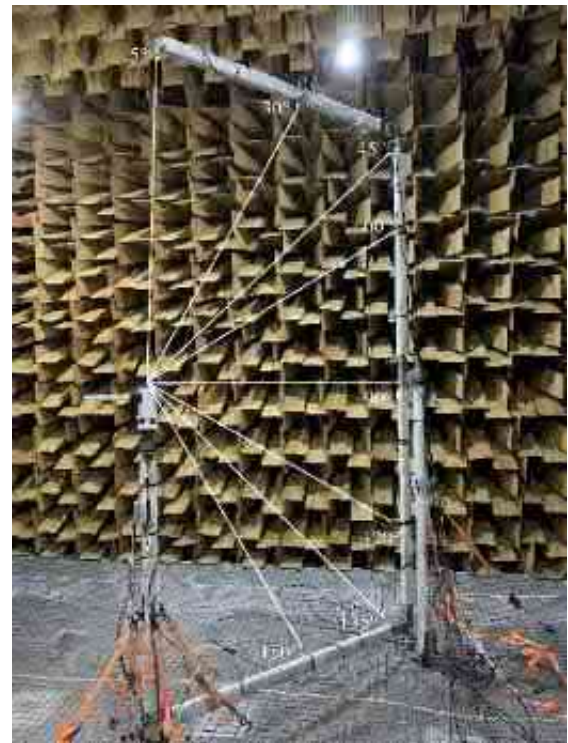
Figure 2: Far-field measurement setup. The polar angles (measured from the propeller axis) of each microphone are shown.
