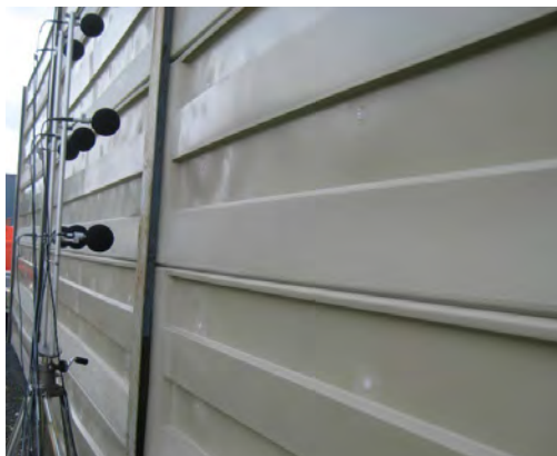
Figure 2: Microphone array in position for in-situ testing
