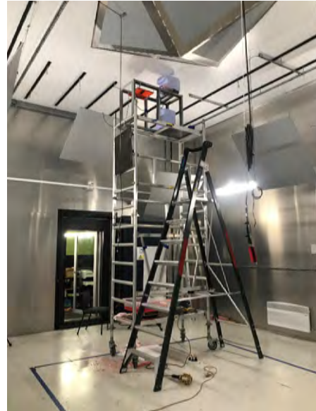
Figure 5: Trial rainfall rig
