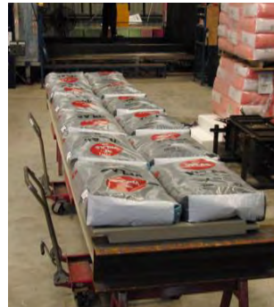
Figure 8: Load testing of a panel
