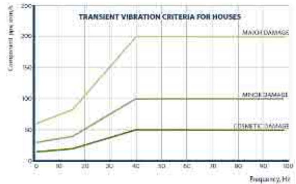
Figure 15. BS 5228-2 criteria (as component ppv mm/s) for short-term (transient) vibration on house structures (4)
