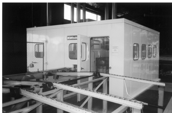
Acoustic enclosure in a timber processing factory
