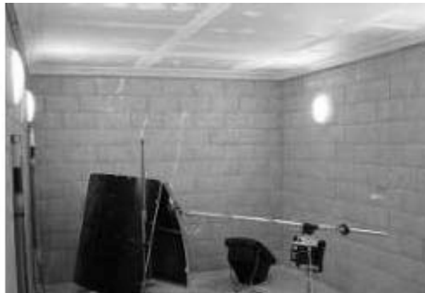
Figure 2, Floor test rig, 200 small Figure 3, Floor Test Rig, End dia. poles @ 600mm centres Measuring the sound field
