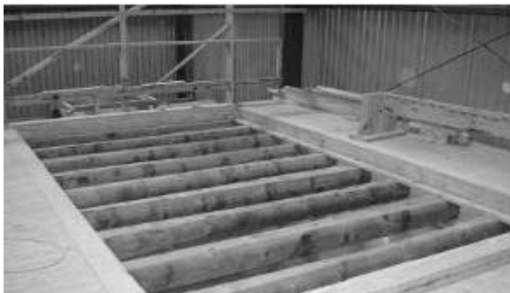
Figure 2, Floor test rig, 200 small Figure 3, Floor Test Rig, End dia. poles @ 600mm centres Measuring the sound field
