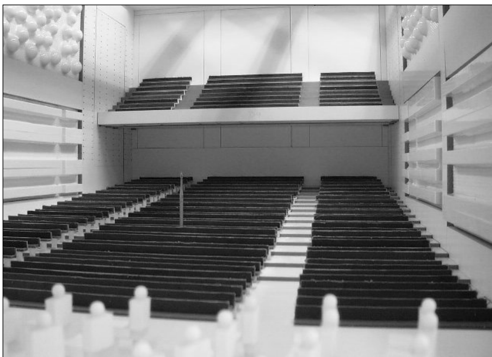
Figure 2 Photograph of the concert hall model with scattering panels on the side walls
