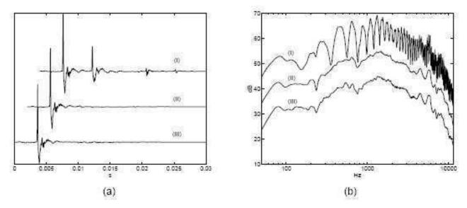
Figure 2. The responses of a loudspeaker found from MLS responses: (I) near a reflecting surface, (II) near a reflecting surface but with the loudspeaker and microphone rotating, and (III) in an anechoic chamber.
