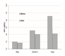
Figure 11: Noise Levels Before and After Control at #2 Due to the Operation of Mill #2 Only
