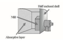
Figure 4: Noise Absorption Layers in the Inner Surface of the Shell
