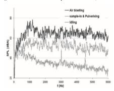
Figure 2: Noise Spectra at #2 When Mill 2# Operates Alone
