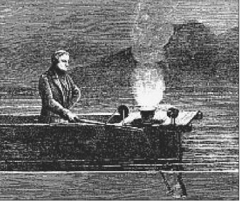
Measurement of the propagation speed of sound in water of the Lake Geneva in 1828 (observation point 1) according Guillemin (1868)
