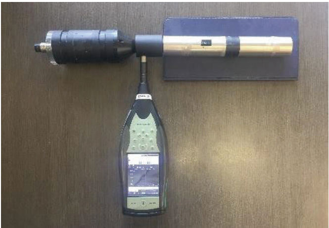
Figure 2. Calibration using a pistonphone
