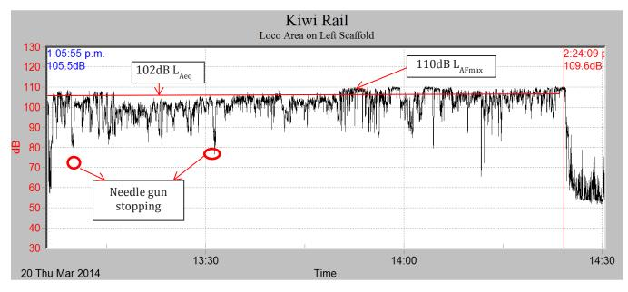
Figure 2: Time History of sound pressure levels in the locomotive panel preparation area
