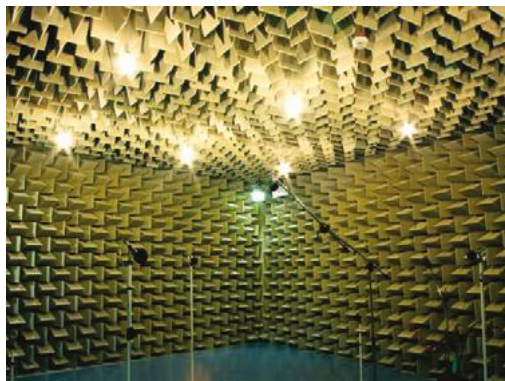
Figure 3. (a) Semi-anechoic chamber and (b) binaural recording set-up
