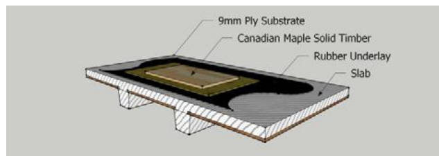
Figure 2. Floor construction schematic
