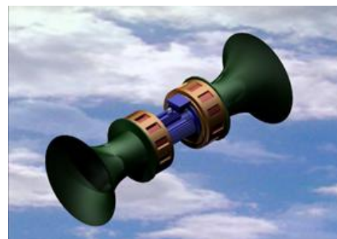
Figure 2: Solidworks image of a 150 dB New Zealand made rotary siren with 45 degree internal reflectors and impedance transformer horns
