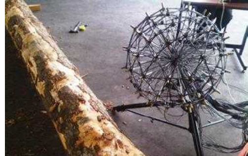
Figure 12: Photo of microphone phase array setup used for field measurements to investigate knot detection imaging
