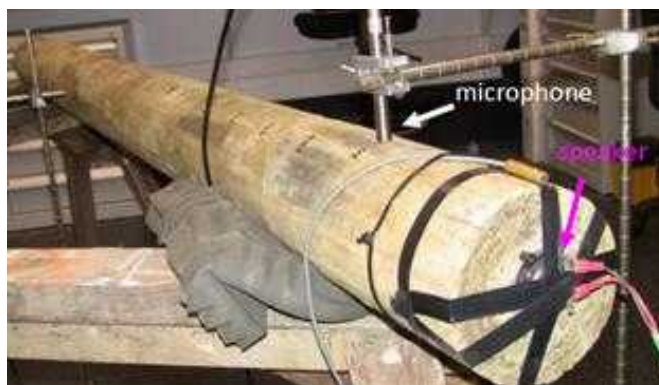
Figure 3: Photo of experimental set-up in the lab for contact microphone measurements
