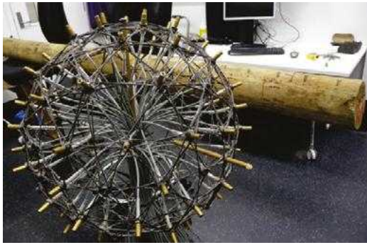
Figure 9: Photo of the microphone phased array experimental setup used in the lab to image the location of knots
