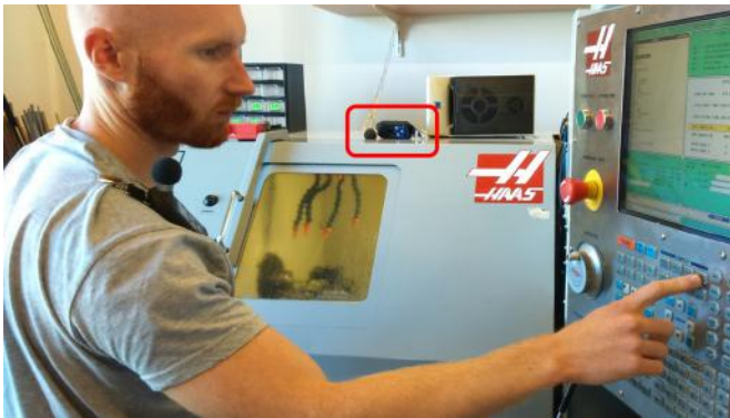
Figure 3: Worker operating CNC machine, left shoulder PSEM detached and positioned on CNC chamber
