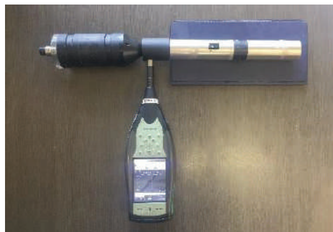
Figure 2. Calibration using a pistonphone
